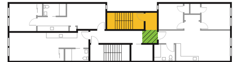
Figure 5 Cutting 1 Stairway and Some Corridor Space Makes a Small Apartment Building Project More Financially Viable Plan of a typical small multifamily building in Jersey City, New Jersey
